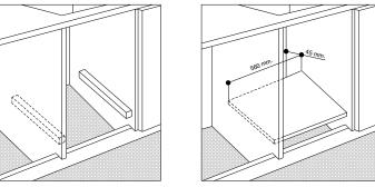
The panels of the adjacent cabinets must be made of heat-resistant material .In particular ,cabinets with a veneer exterior must be assembled with glues which can withstand temperatures of up to 100°C.
